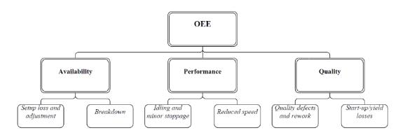
In the packaging industry, it is well known that accumulation is widely used to reduce the idling and minor stoppages expected in a production line. (Parker, 2018)
