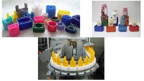
Many containers however are less complex as they are flat based, stable and easier to handle as shown below but due to the characteristics of the product being filled, i.e. highly viscous or containing solids, they are often filled at much lower speeds of between 8,000 – 15,000 containers per hour.
