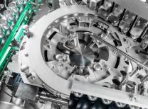
For higher overall line availability, star wheels and guides are built in light-weight sectors for easy and quick replacement, with changeovers possible in less than 30 minutes.
