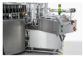
With its stainless-steel structure and components, the EvoDECO Cold Glue labeller is hygienically designed and fully washable.
