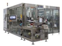
The modular Sidel Matrix<sup>™</sup> SL70 primarily uses wraparound roll-fed technology
