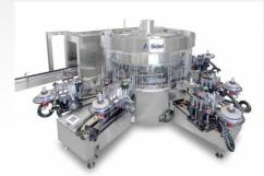
The Sidel SL90 high-speed rotary labeller is able to switch quickly between self-adhesive and cold-glue labels
