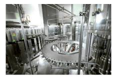
The Sidel Matrix<sup>™</sup> Combi system integrates the blow-fill-cap function in one single enclosure, with neck-handling and positive transfer of PET bottles.
