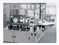
The reel stand of the Rollquattro Evolution has been structurally integrated into the label station to save space
