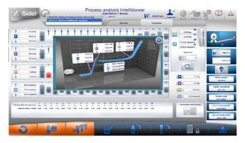
The Sidel Intelliblower<sup>™</sup> eliminates inconsistencies of material distribution by analysing and controlling the blowing curve on each individual PET bottle.
