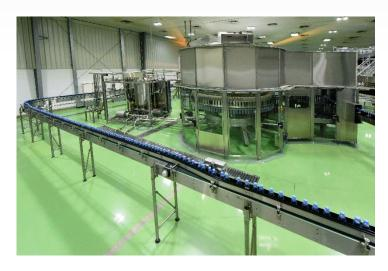
Following the successful installation two years ago of what was Sidel's fastest bottling line in the world at the time, the Health Water Bottling Company (HWB) of Saudi Arabia decided to invest in two further lines. The original solution still runs at a speed of 134,000 bottles per hour (bph), whereas the two new Sidel complete PET water lines are both now running even faster - at the new, record-breaking output rate of 150,000 bph each, making a total installed output of 300,000 bph.
