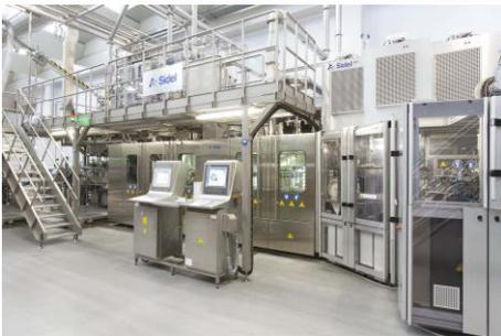
**Centrale del Latte di Brescia has doubled its aseptic production of UHT milk in PET bottles and in doing so is benefitting from a simple, safe and sustainable packaging line. The project saw this innovation-driven company become the first producer in Italy to invest in Sidel's aseptic and environmentally friendly combined blow-fill-cap solution with dry preform decontamination – the Sidel aseptic Combi Predis™.**
