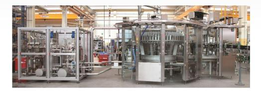
Sidel, the international supplier of liquid packaging solutions to the drinks industry, has produced a new modular hotfill machine that offers customers an extensive range of possible configurations. Part of the Sidel Matrix<sup>™</sup> range, it provides the highest standards of hygiene to meet the production demands of more natural and fresher beverages, even those including pulps or fruit pieces.
