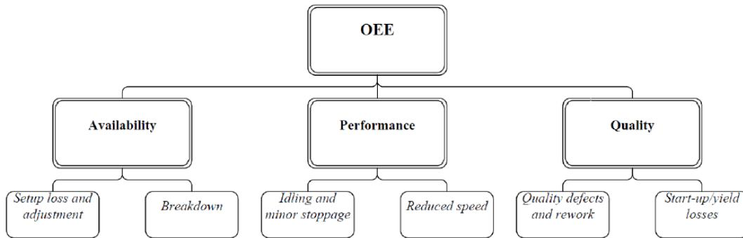
In the packaging industry, it is well known that accumulation is widely used to reduce the idling and minor stoppages expected in a production line. (Parker, 2018)
