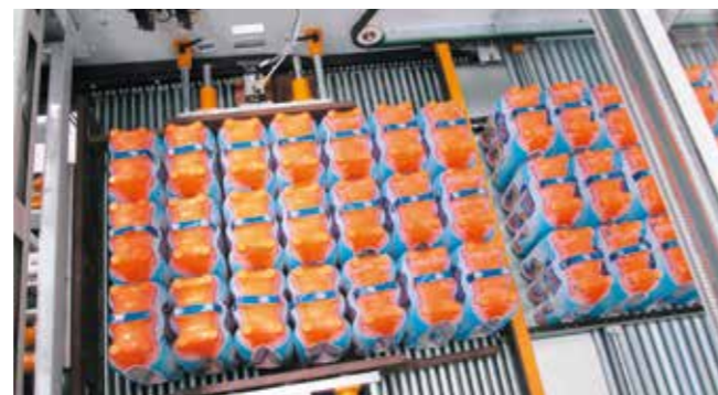
Layer compacting area
