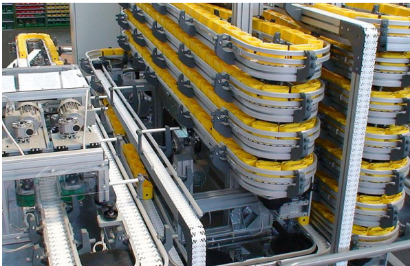
Figure 8 Flexlink balancing conveyors
