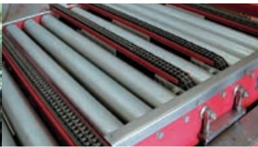
Pallet transfer tables allow change in the orientation and direction of pallet transport.
