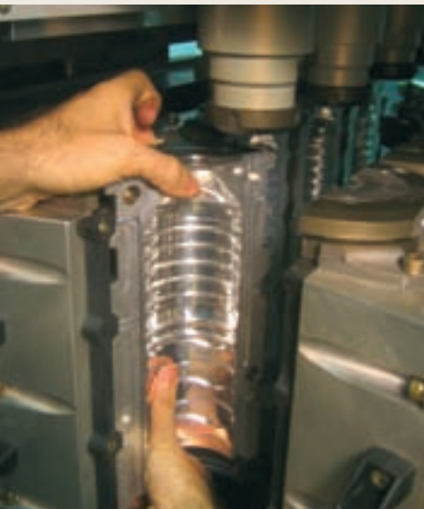
For an SBO 4 Compact, it takes only 15 min for an operator to switch from one production to another (same neck).
