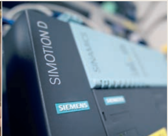
SBO Compact™ equipment incorporates Simotion technology from Siemens. This system controls all machine movements 1,000 times per second with precision down to .10/mm. The system offers total flexibility in operating virtual cams.
