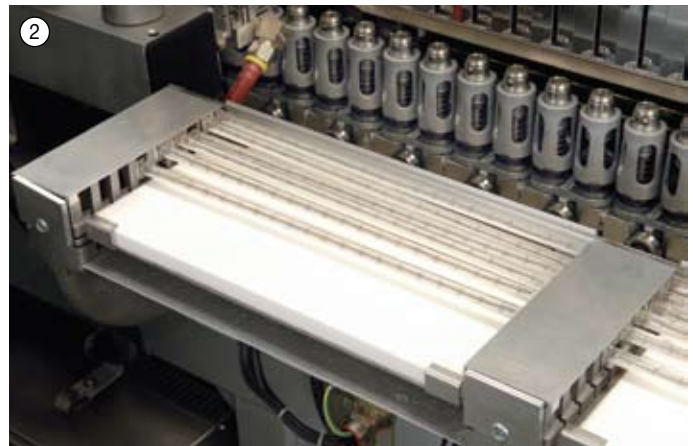
Passage of preforms in the blow molder oven
