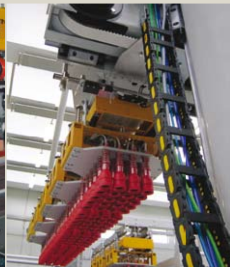
Brushless head motorization with toothed drive belts
