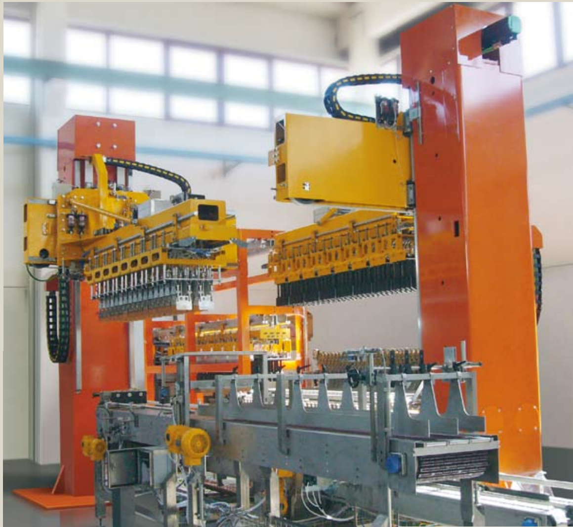
Double crater for bottles and cluster pack application
