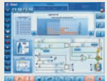
The electrical consumption is displayed in the HMI (Human Machine Interface) window.
