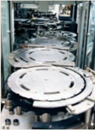
The Combi concept is built on highly reliable rotary kinematics and perfectly synchronized blow molding and filling.
