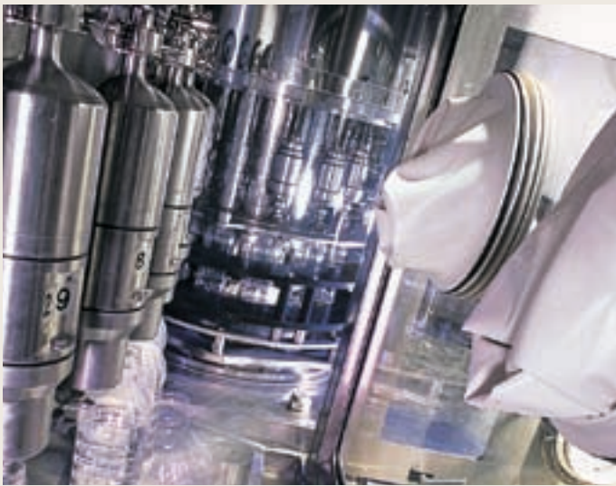
The Combi can be equipped with glove boxes to service the machine without opening it.
