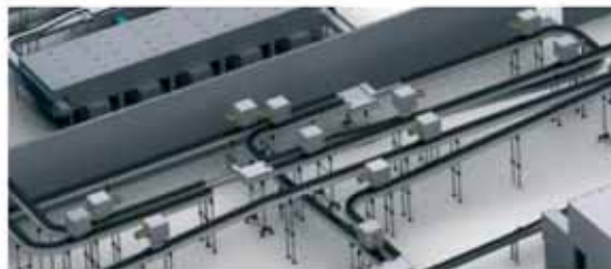
High-speed air conveyor switching systems for multi-product and multi-format lines.
