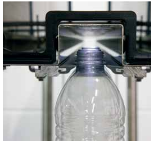
Friction coefficient, format changeover, maintenance: we pay special attention to your bottle's neck guide rail.
