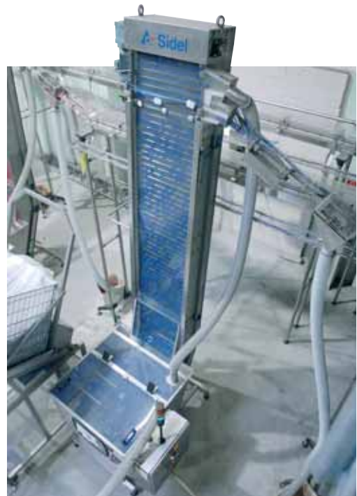
Remote feeding outside the filling area.
